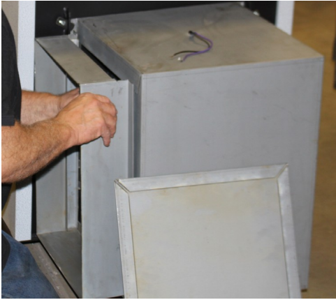
Installing Filter Rail
